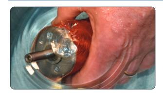
**STEP 5.**If leak is in bladder you will need to replace the bladder.
