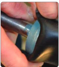
**STEP 6.**If bladder is leaking, disassemble the unit using the Philips screwdriver.
